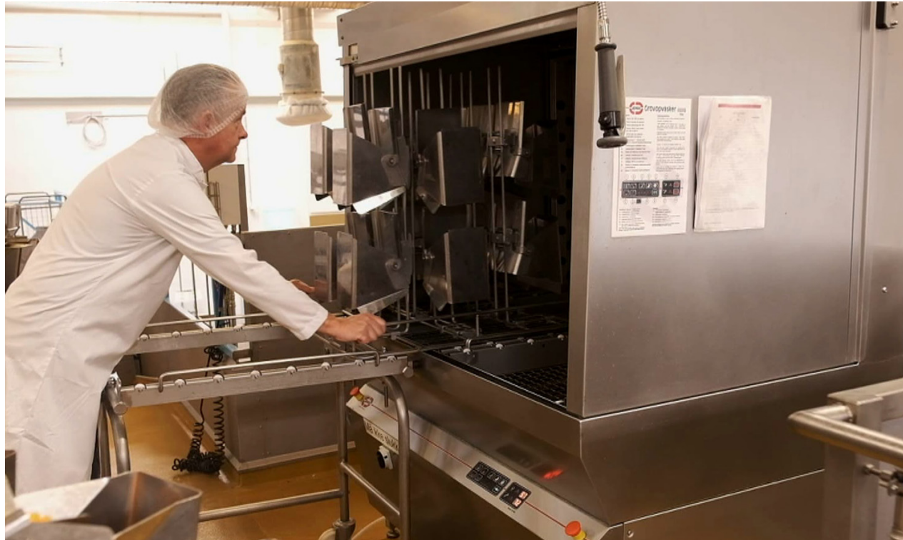
JEROS' machines take advantage of a washing frame that runs back and forth, where turbines first wash the items at 52 degrees and then rinse them with water at 85 degrees. It ensures that there is no listeria, salmonella or other bacteria that can spread from the washed items to other areas of production.
