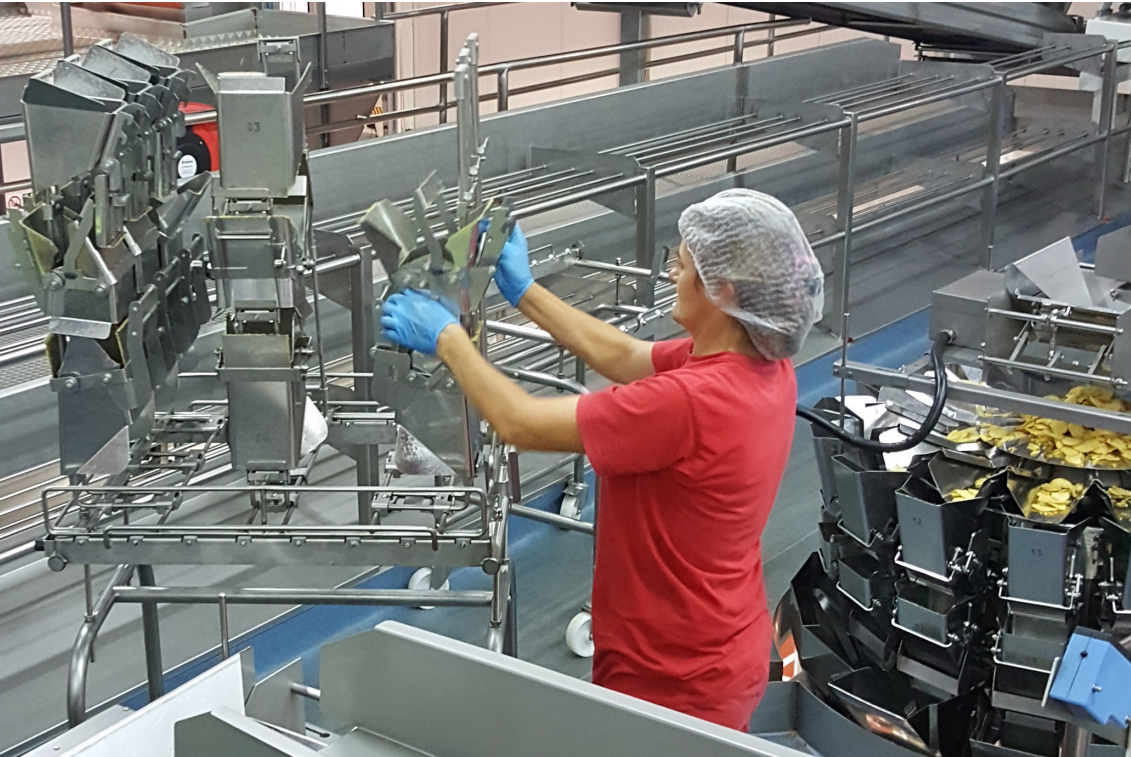
JEROS has developed a variety of trolleys and racks where the user can place dismantled components and transport them, for example, scale pans. With JEROS solutions it is possible to wash up to 48 scale pans within 3-6 minutes. Photos: JEROS
